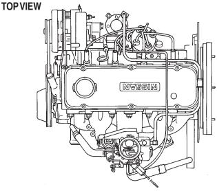
Figure 9. Nissan Model A15 Basic Engine Components
